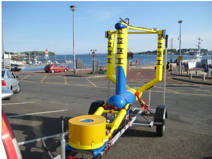
Figure 1: Evopod ready for slip launching
